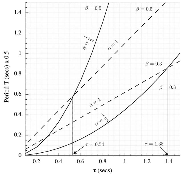
**Fig. 2** Plot of period  $T$  versus  $\tau$  to two values of  $\beta$  for the multivibrator. The dashed line represents  $\alpha = 1$  or the result with a normal capacitor and the solid line represents the result due to the fractional capacitor  $\alpha = 0.5$
