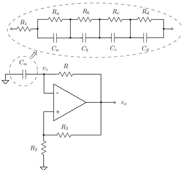
**Fig. 1** The free running multivibrator with fractional capacitor  $C_x$ . In the inset a RC realization of the fractional capacitor  $C_x$  using the method of [1]
