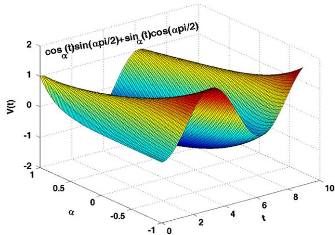
Figure 4. 3D plot of the voltage  $V(t)$  across a fractance device excited by a sinusoidal current.
