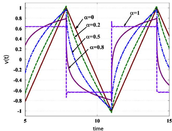
Figure 5.  $V(t)$  across a fractance device for different  $\alpha$ 's if  $I(t)$  is a triangle waveform obtained from numerical integration of (8).
