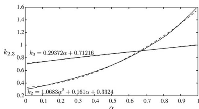
**Figure 3** Plot of  $k_2$  and  $k_3$  against  $\alpha$  that yields minimum passband error in (5) and the interpolated functions as solid and dashed lines, respectively
