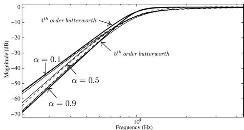
**Figure 9** MATLAB simulation and FPAA experimental results of the magnitude response of the approximated  $(4 + \alpha)$  order FHPF, shown as solid and dashed lines, respectively, compared against the fourth- and fifth-order standard Butterworth high-pass filters
