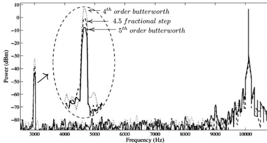
**Figure 10** Frequency spectrum of the approximated 4.5 order FHPF (dashed) compared to fourth (dotted) and fifth (solid) order high-pass Butterworth filters
