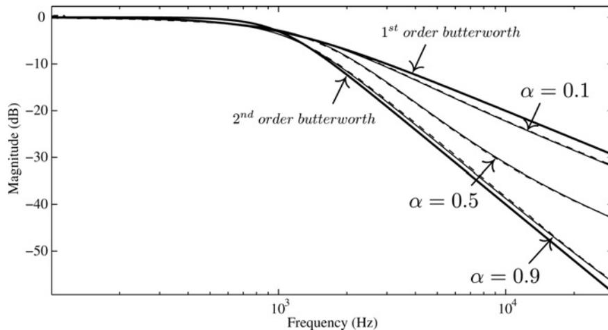
**Figure 6** MATLAB simulation and FPAA experimental results of the magnitude response of the approximated  $(1 + \alpha)$  order FLPF, shown as solid and dashed lines, respectively, compared against the first- and second-order standard Butterworth low-pass filters
