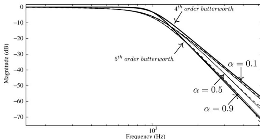
**Figure 7** MATLAB simulation and FPAA experimental results of the magnitude response of the approximated  $(4 + \alpha)$  order FLPF, shown as solid and dashed lines, respectively, compared against the fourth- and fifth-order standard Butterworth lowpass filters
