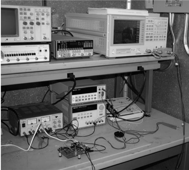
**Figure 5** Test setup to measure the magnitude response of circuits implemented on the AN231E04 with a HP4395A network analyser
