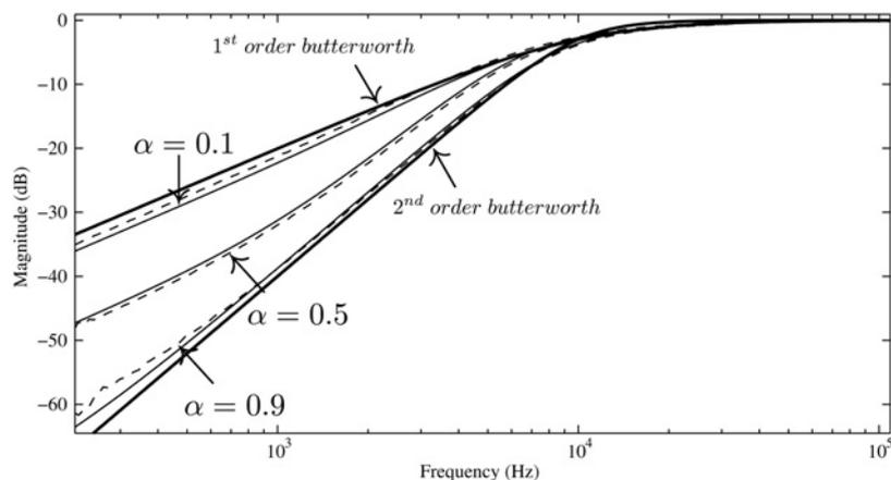
**Figure 8** MATLAB simulation and FPAA experimental results of the magnitude response of the approximated  $(1 + \alpha)$  order FHPF, shown as solid and dashed lines, respectively, compared against the first- and second-order standard Butterworth high-pass filters
