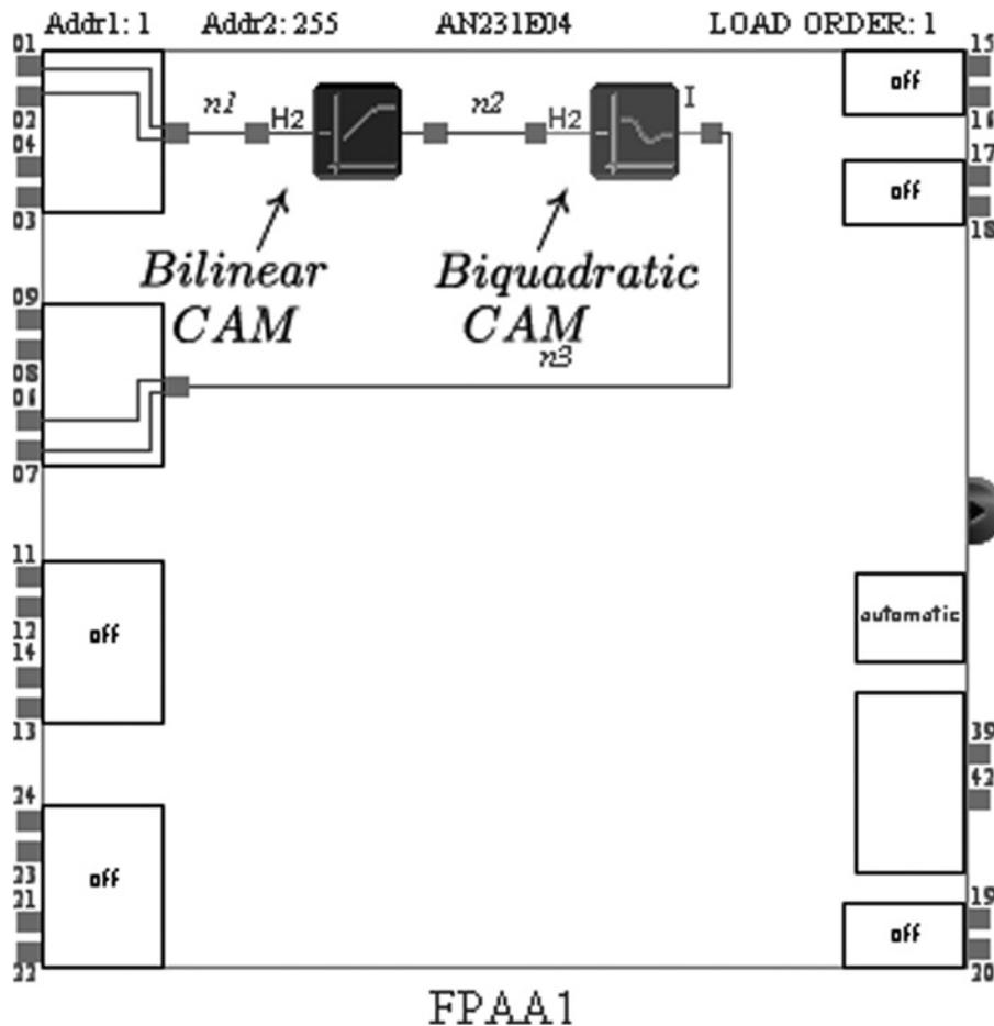
Figure 4 Cascaded connection of the bilinear and biquadratic filter CAMs in the AnadigmDesigner environment
