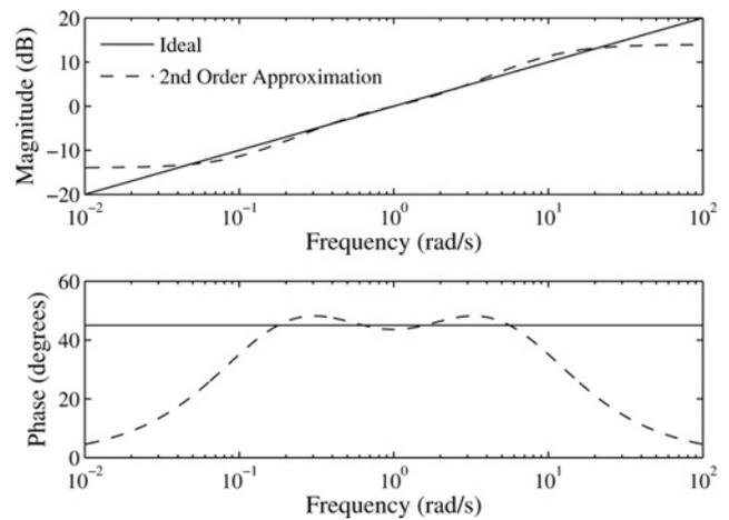
**Figure 2** Magnitude and phase of  $s^{0.5}$  using second-order approximation (dashed) compared to ideal case (solid)
