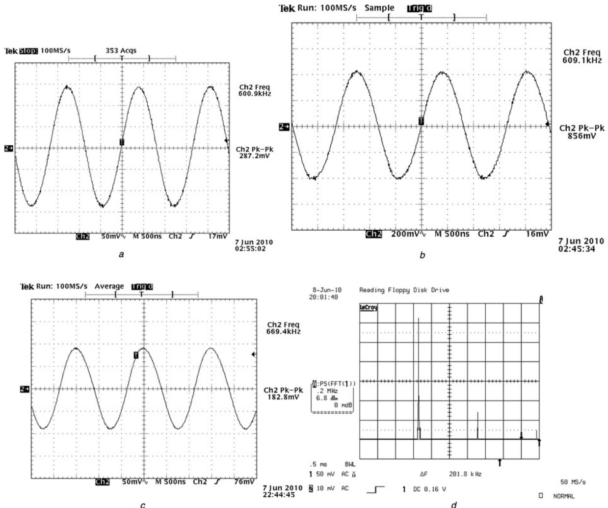
Fig. 4 Experimental waveforms of the voltage across  $C_2$  for the oscillator in Fig. 3 at
