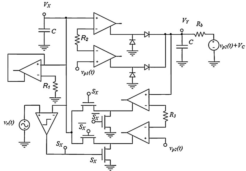
Fig. 2. Circuit for experimental verification. All op amps are AD844s. MOS transistor switches are LM4066.
