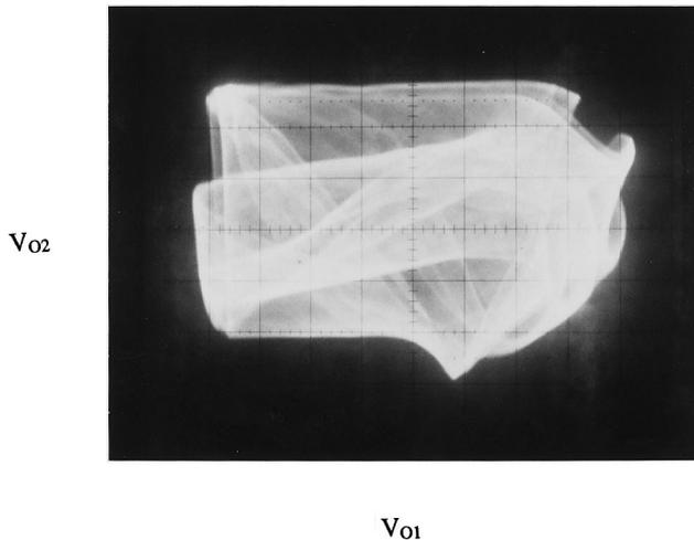
Fig. 4. Experimentally observed  $V_{01}$ – $V_{02}$  trajectory. X-axis: 0.2 V/div; Y-axis: 0.2 V/div.
