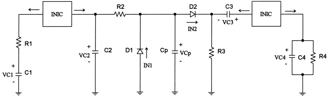
Fig. 1. The new hyperchaos generator.
