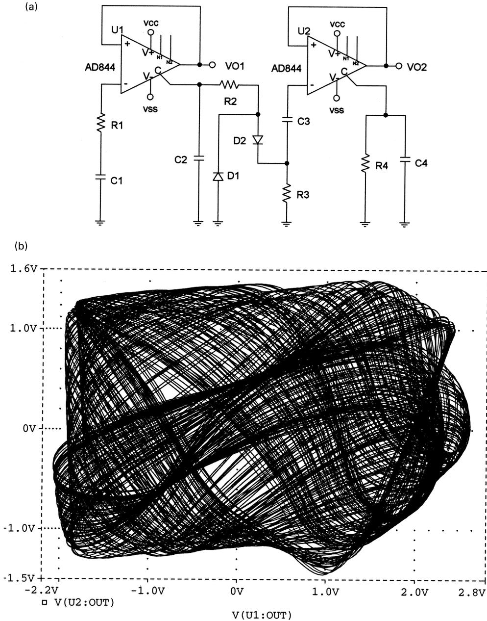
Fig. 3. (a) A circuit implementation of the hyperchaos generator using AD844 CFOAs; (b) PSpice simulation representing the  $V_{O1}$ – $V_{O2}$  chaotic attractor.
