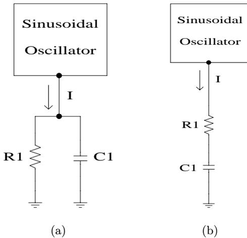
Fig. 1. Class of sinusoidal oscillators with (a) a parallel RC network, (b) a series RC network.
