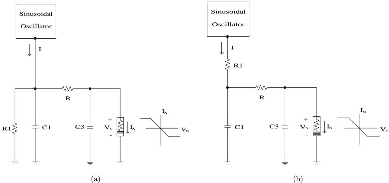
Fig. 2. Chua's circuit based on the oscillator (a) in Fig. 1(a), (b) in Fig. 1(b).
