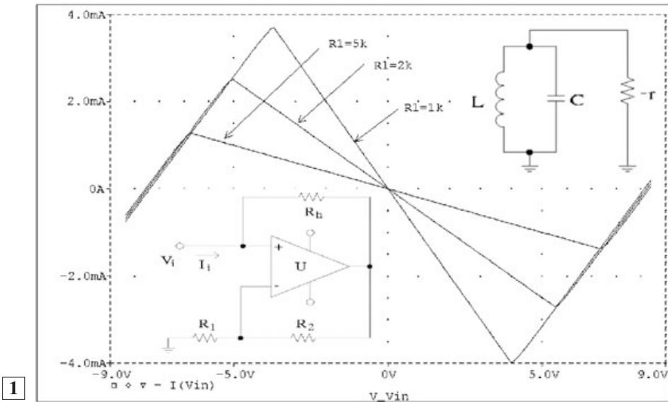
Fig. 2 Active tank oscillator (upper right) using a voltage-controlled negative resistor (lower left) and PSpice d.c. simulation of its characteristics ( $R_2 = R_n = 1\text{ k}\Omega$ ,  $\pm 9\text{ V}$  supplies).
