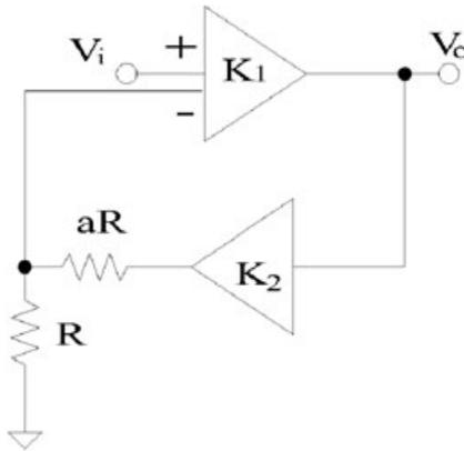
Fig. 4 Proposed two-amplifier structure for realising 3-segment nonlinear characteristics.
