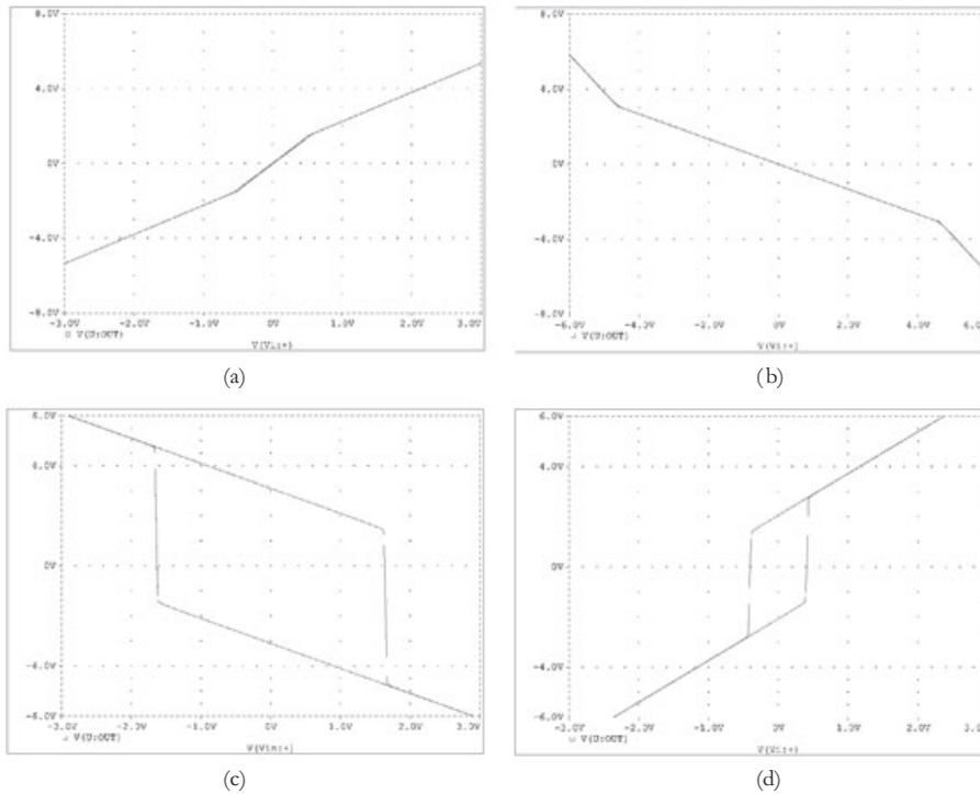
Fig. 5 PSpice simulations of the obtained nonlinear characteristics of Fig. 4 using op-amp based amplifiers biased with  $\pm 7V$  supplies; (a)  $(K_1, K_2, a) = (2, -1, 3)$ , (b)  $(K_1, K_2, a) = (-4, 1, 1)$ , (c)  $(K_1, K_2, a) = (-4, 1, 4)$ , (d)  $(K_1, K_2, a) = (-2, -2, 2)$ .
