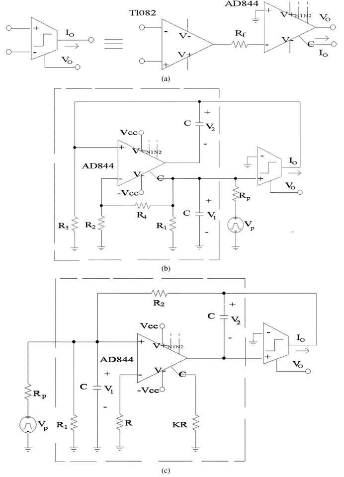
Fig. 4. Circuit realizations of (a) the nonlinear transconductor, (b) a chaotic oscillator based on the single resistance controlled oscillator of [17], and (c) chaotic oscillator based on the Wien bridge oscillator.
