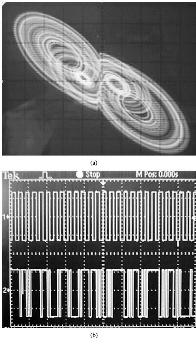
Fig. 5. Experimental observations representing (a) the  $V_{C1} - V_{C2}$  phase-space projection for the circuit in Fig. 4(b) ( $X$  axis: 0.5 V/div,  $Y$  axis: 0.5 V/div) and (b) sample of the periodic input and chaotic output pulse time waveforms for the circuit in Fig. 4(c).
