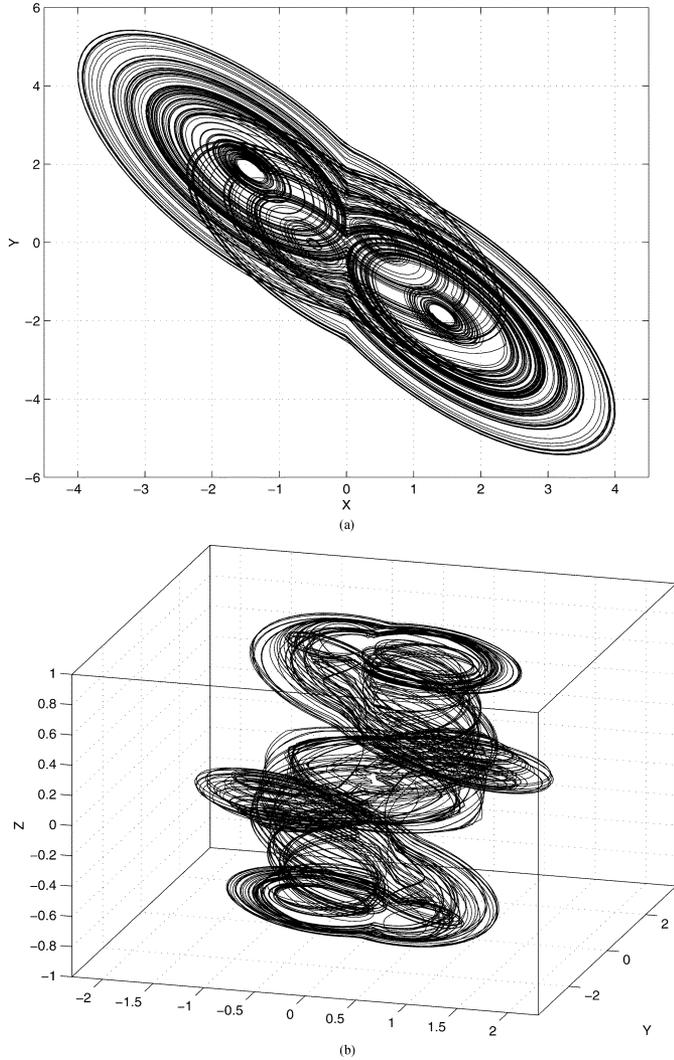
Fig. 2. Chaotic attractor obtained from (6) with  $(\varepsilon, n, \beta, \phi) = (0.05, 1, 0.5, 0.2)$ . (a) Projection in the  $X$ - $Y$  plane and (b) constructed 3-D view by using (1) in conjunction with (6).
